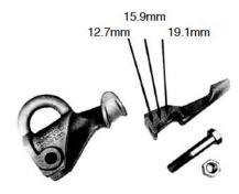
1. Component Parts: The keeper is to be used with 12.7mm, 15.9mm, and 19.1mm anchor rods (see arrows). For 25.4mm and 31.8mm anchor rods, the PREFORMED Pulling Eye is used without the keeper.
