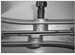
**PLP Tip:** Tightening the bolt slightly by hand will prevent the frame halves from moving apart.
