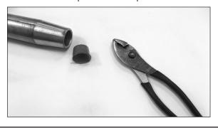
**Step #3** Measure the length of the aluminum splice body.
