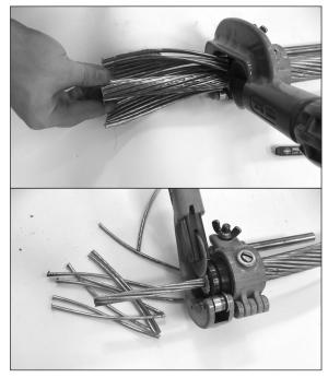
**PLP TIP:** To ensure no damage to the steel core and for rapid installation, PLP recommends the use of a Utility Approved Trimming Tool. After the strands are removed, any flash or burrs on the outside can be removed with a file.
