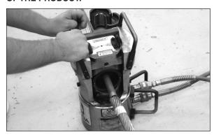
PRECAUTION: TO BE A CORRECT APPLICATION, COMPRESSION CURVATURE MUST BE KEPT TO A MINIMUM, PREFERABLY LESS THAN 1/2 THE ALUMINUM TUBE DIAMETER FROM THE CENTERLINE. FOR THE STEEL, CURVATURE SHOULD NOT BE VISIBLE. EXCESSIVE COMPRESSION HARDWARE CURVATURE IS A MISAPPLICATION OF THE PRODUCT.
