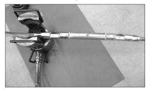
NOTE: The section of the tube marked "DO NOT PRESS" should not be compressed.
