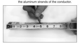
Step #6 Apply tape approximately 1" back from the cutting mark to secure the aluminum strands and maintain the conductor diameter after the cut is made.
