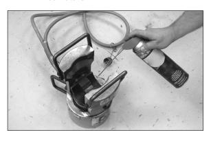
Step #15 Insert the assembly into the compression press on one side of the "Press First" knurl. After, ensure that the proper alignment of the steel core splice tube is still maintained with both pieces of the conductor remaining properly inserted into the splice tube.
