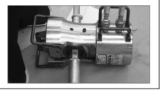
Step #27 Once the first piece of conductor is compressed, move the press back to the "Press First" knurl and repeat the aluminum splice body compression process for the other conductor piece.
