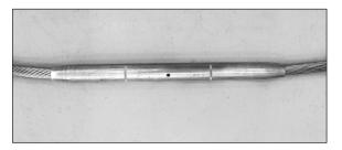
NOTE: The tapered ends of the aluminum splice body should be at the marks made earlier, indicating that the splice is centered over the two conductor sides. FAILURE TO PROPERLY CENTER EITHER THE STEEL OR ALUMINUM SPLICE TUBES IS A MISAPPLICATION OF THE PRODUCT.
