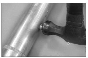
**Step #24** Peen over the aluminum edges of the filler hole with a hammer and flat head screwdriver to secure the ball into place.
