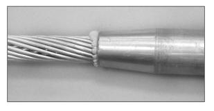
**Step #22** Seal the filler hole by inserting the stainless steel ball.
