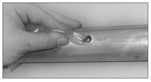
**PLP TIP:** The plastic bag containing the ball should be used to more easily position the ball into place than by hand and to avoid dropping the ball.
