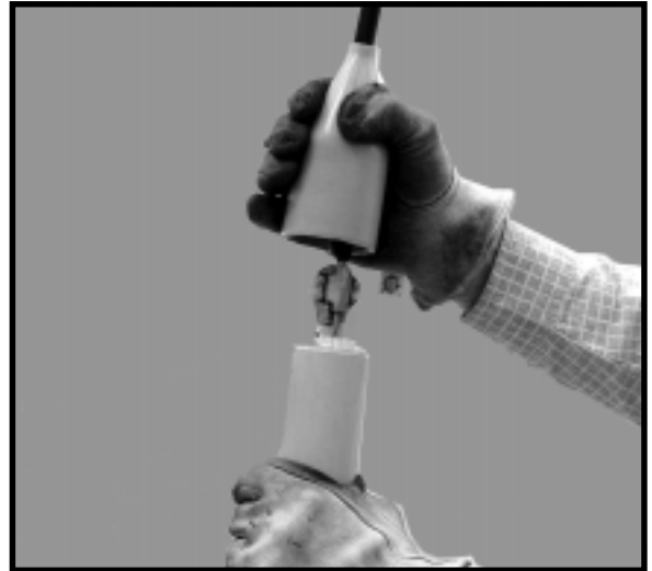
FIGURE 10 - Installation of tip/nose
