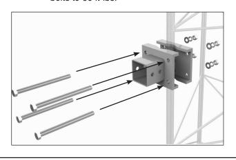
Step #3 Install the lower tower mount. Once the upper and lower tower mounts are installed, the main antenna mount structure is ready to be installed.
