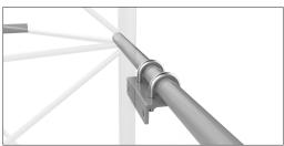
Step #13 Attach the two 1/2" bolts to the tie back and V-Backing Plate. Then attach the tie back assembly to the tower. Ensure the two U-bolts and the two 1/2" bolts are torqued to 30 ft-lbs.
