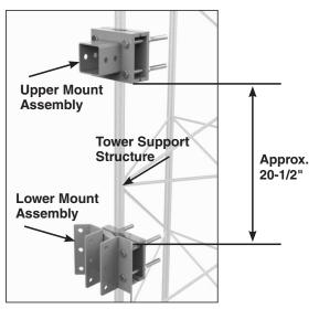
**PLP Tip:** If the tower support structure is impeding the installation on the lower mount assembly, it can be adjusted up 3" or down 3" on the tower support leg.
