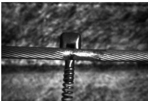
Figure 4 – Abrasion Damage at Spacer
