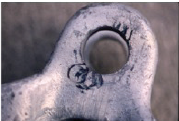
Figure 22: Suspension housing damage due to galloping
