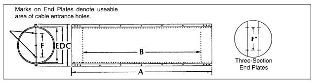
\*Spacing of ¼" required between holes drilled along the seams of two and three section end plate in the "usable area".
