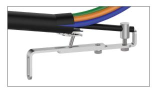
Step #9 Secure the strength member in the retention housing by tightening the bolt. Secure the shield connector to the bracket assembly with the nut provided with the shield connector.
