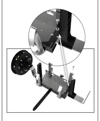
Step #4 Secure the deep metal transition tray to the organizer bar with the two plastic washers and two combination head screws provided in the replacement kit (P/N: 80061335). This connection should be hand tight.
