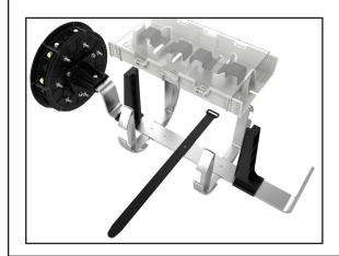
Step #3 Place the deep metal transition tray from the replacement kit (P/N: 80061335) on the organizer bar, in the same location where the plastic transition tray was originally.
