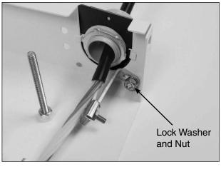
**Step #16** Slide the adapter port nut halves apart as shown below.
