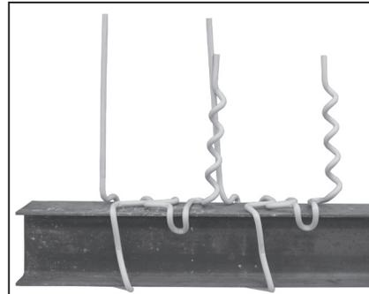
**Step #5** Wrap the helical upright of the first deterrent around the straight upright of the second deterrent. Ensure that the bottom helical wrap is installed properly.
