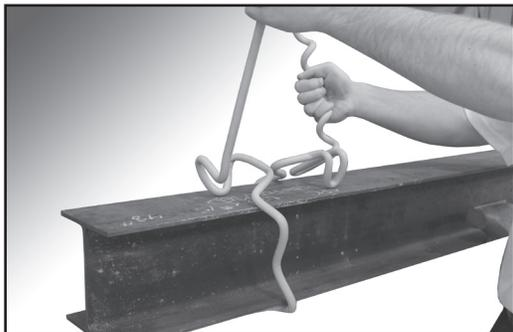
**Step #3** Lifting on the uprights, flex them away from each other to snap the hooks over the top edges of the I-Beam.
