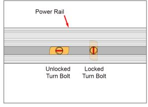
Insert 5/16" x 3/4" Turn Bolt into Power Rail and rotate 90-degrees, locking Turn Bolt in place. On the outermost "L" Feet align center of the "L" Foot with the
