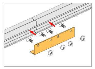
Splice Plates come in two configurations, 2-hole or 4-hole (above is a 4-hole). Insert 5/16" x 3/4" Turn Bolts into Power Rail and rotate 90-degrees to lock
