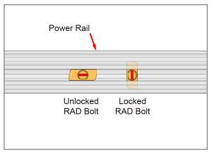
AMP Clamp bonding Mid Clamps are inserted into the Power Rail and positioned between adjacent Modules. Insert the 5/16" RAD Bolt into Power Rail and rotate
