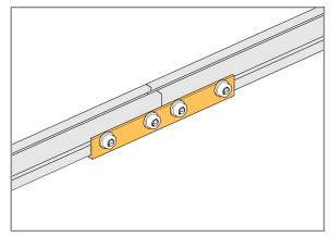
Turn Bolts in place. Align Splice Plate with center of splice and secure to Power Rail with 5/16" Flange Nuts. **Torque to 15 ft.-lbs.**
