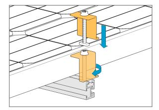
RAD End Clamps are used on the outer Modules. Insert the 5/16" RAD Bolt into Power Rail and rotate 90-degrees clockwise to lock the RAD Bolt within the Power Rail. Secure with 5/16" Flange Nut. **Torque to 15 ft.-lbs.**
