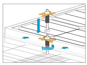
90-degrees clockwise to lock the RAD Bolt within the Power Rail. Push Modules against AMP Clamp. Tighten 5/16" Flange Nut. **Torque to 15 ft.-lbs.**
