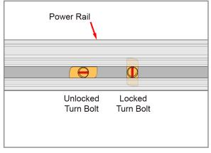
Insert 5/16" x 3/4" Turn Bolt into Power Rail and rotate 90-degrees, locking Turn Bolt in place. On the outermost "L" Feet align center of the "L" Foot with the
