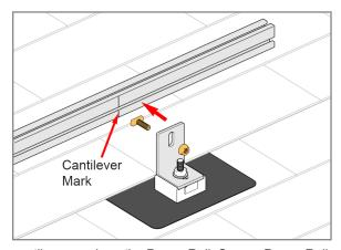
cantilever mark on the Power Rail. Secure Power Rail to "L" Foot with 5/16" Flange Nut.
