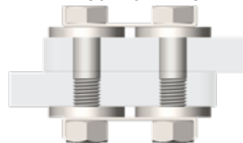
Fig D S/S BOLTS AND NUTS WITH LARGE SERIES WASHERS AND LOCKING PLATES
