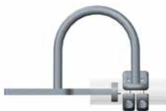
Busbar temperature = 20^{\circ}\text{C} (As Installed)
