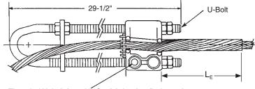
Threaded Hole (1/2-13 UNC, 7/8" deep) to fit class 2A Galvanized Bolt for Grounding Connection.
