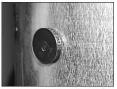
The POLE PLUG is designed to close an existing hole in a steel structure in order to reduce whistling and prevent insect intrusion. It provides an economical means of reducing insect and wildlife nesting which can disturb linemen while working on the lines. Pole Plugs are available in 9/16" to 3". Please consult PLP's Energy Catalog, for catalog numbers or PLP for custom sizes.
