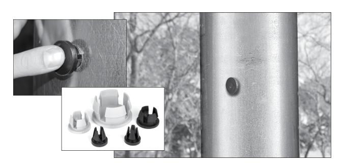
The POLE PLUG is designed to close existing holes in steel and composite utility poles or other equipment in order to reduce or eliminate whistling due to the wind and insect intrusion. The plug provides an economical means of reducing the incidents of insect infestations. This reduces possible injury to lineman and loss of productivity.
