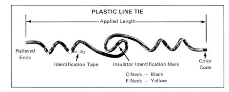
Plastic Line Ties are intended for use on "tangent" construction with jacketed conductors and vertically mounted tie top insulators on cross-arms, pole-top mounted insulators, or Spacer Cable brackets. Line angles of up to 15° are recommended.
