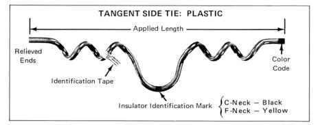
Plastic Tangent Side Ties are intended for use on "tangent" construction with jacketed conductors and side mounted tie top insulators on armless construction.Line or sag angles of up to 15° are recommended.
