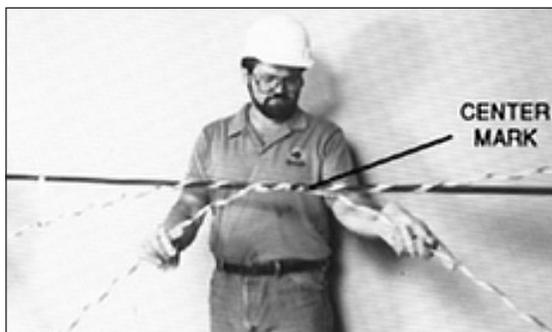
**STEP 4** Wrap the second subset on the cable for two or three pitch lengths, leaving the ends loose, as shown below.
