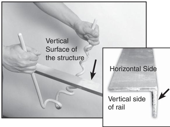
**Step #3** Rotate the Bird Perch Deterrent 90° clockwise in the horizontal plane and position the diverter where desired.
