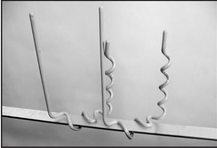
**Step #7** Continue wrapping the helical leg until it is completely installed.
