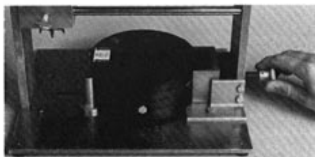
FIGURE 8 - PLACING END PLATE IN CUTTER
