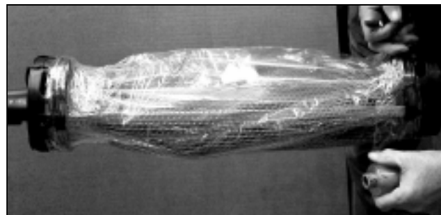
FIGURE 7 - USE PRESSURE WRAP TAPE TO SEAL ENDS OF LINER ON END PLATE
