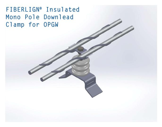
The clamp body is made from aluminium alloy, and is designed to clamp onto the angle iron member of steel towers, and to secure OPGW downleads to structures while minimising compressive clamping forces which could be transferred to the optical elements.
