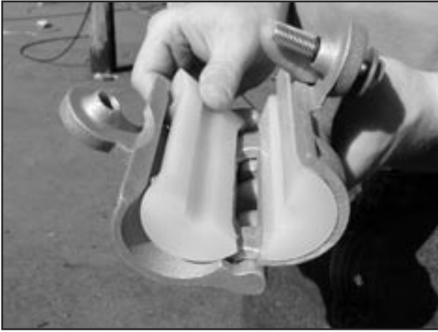
FIGURE 8: UNGRITTED CUSHION INSERTS IN OPEN KEEPERS
