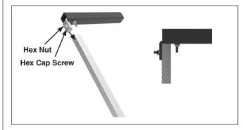
**STEP #4** Completed installation of the Perch onto the RAPTOR PROTECTOR™ Platform.
