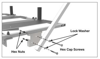
STEP #3 Install the perch crossarm by sliding the preinstalled hex cap screw into the slot of the support leg. Tighten the hex nut to secure the crossarm in place.
