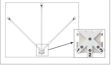
**NOTE:** The perch installs into the same position as one of the Nest Retention Posts.
