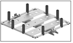
Step #3 Secure the platform to each pole top bracket with (2) carriage bolts, (2) flat washers, (2) lock washers, and (2) hex nuts as shown below. Go back and fully tighten the 5/8" through bolts (shown in Step #1).
