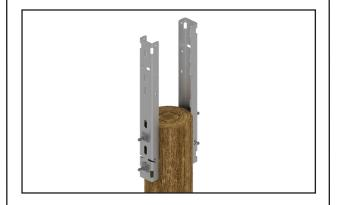
Step #2 (OPTIONAL) If using the optional nest retention posts, attach each nest retention post to the platform frame using a nylon lock pin. Push the pin all the way through the pre-drilled hole from the outside of the frame toward the inside.
