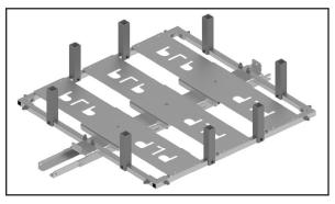
Step #4 Mount the pole channel using stainless steel straps or 5/8" through bolts and flat or square washers, (Not supplied).
