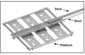
**Step #2** Ensure that the struts are oriented as shown below.
