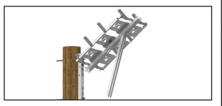
**Step #6** Slide the ends of the struts into the slots on the pole channel as shown below.
