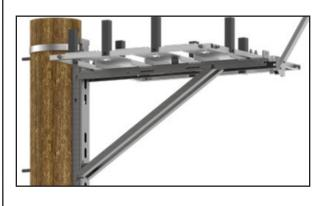
Step #7 Secure the platform to the pole channel using (2) hex head bolts, (4) flat washers, (2) lock washers and (2) hex nuts. Fully secure the struts to the platform at this point.
