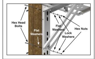
Step #8 Completed installation of the RAPTOR PROTECTOR™ Nesting Platform shown below.
