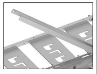
Step #3 (OPTIONAL STEP) If using the optional nest retention posts, attach each nest retention post to the platform frame using a nylon lock pin. Push the pin all the way through the pre-drilled hole from the outside of the frame toward the inside.
