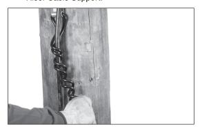
**Step #2** Tighten the lag bolt to secure the Riser Cable Support to the utility pole.
