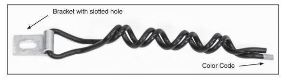
**Step #1** Pre-drill a hole into the utility pole and insert a lag bolt through a washer and through the slotted hole in the bracket.
