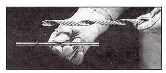
10.00 When using the subset method of installation it is necessary to place a pin or dowel inside the subset to hold it in proper position.
