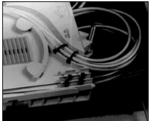
FIGURE 13 - SECURE TUBES TO SPLICE TRAY
