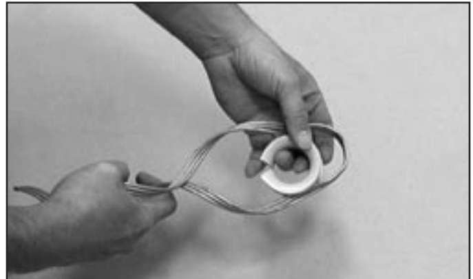
FIGURE 8: OPENING UP THE LOOP AND INSTALLING THIMBLE
