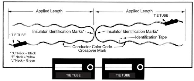
**Tie Assembly:** A Double Side Tie assembly consists of two metal tie components plus two tie tubes.
