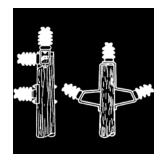
LINE ANGLES GENERAL GUIDELINES: On horizontally-mounted insulators, Alloy Side Ties can normally accommodate line angles up to 10°. On vertically-mounted insulators, line angles up to 40° can normally be achieved. When insulators are mounted at various degrees of cant between the horizontal and the vertical, line angles between 0° and 40° may be accommodated depending upon the actual cant of the insulator.
