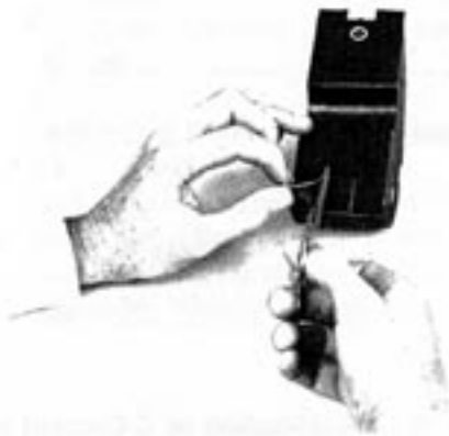
Figure 20 — LOCK-TAPE™ Sealant Application to End Plate Half.
