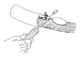
3. Once in position, slide the thermal pair protector under the base plate of the connector assembly to isolate the connector from the cable core wrap.
