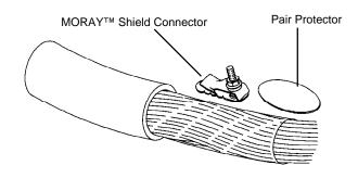
2. Slide the connector with thumb pressure into the cable sheath opening. If you cannot easily slip connector in, then follow tip below.
